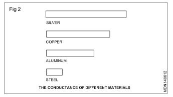
Since different metals have different conductance ratings, they must also have different resistance ratings. The resistance ratings of the different metals can be found by experimenting with a standard piece of each metal in an electric circuit. If you cut a piece of each of the more common metals to a standard size, and then connect the pieces to a battery, one at a time, you would find that different amounts of current would flow. (Fig 3)
