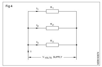
In a parallel circuit, individual branch resistances offer opposition to the current flow though the voltage across the branches will be same.
