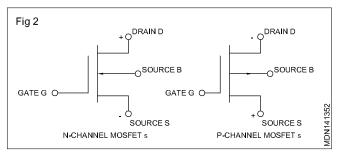
N-Channel MOSFETs are operated with a positive drainsource Voltage. They have a considerably greater practical significance than p-channel MOSFETs, which require a negative drain-source voltage for their operation.
