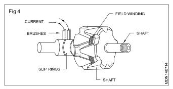
This consists of a steel shaft which carries the driving pulley and cooling fan, a cylindrical iron core, and two stationary part which is held between two end covers. (Fign 5)
