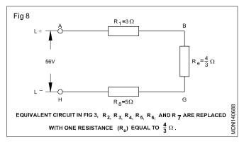
The total combined resistance of the circuit is  $9\frac{1}{3}$  ohms.
