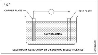
Copper and Zinc in salt solution is one combination
