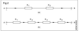
The lamps are replaced by resistors in Fig 2. Fig 2 (a) shows two resistors are connected in series between point
