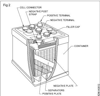
**Construction:** The automobile battery's plates are rectangular. They are made of lead. Antimony alloy is used to provide them strength.
