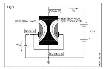
If the main current flow is only through the N-doped material, then such a FET is reffered as a P-channel or P type FET. The current through the P-doped material in the P-type FET is only by Holes.
