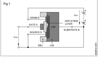
Here, two highly doped n-zones are diffused into p-doped silicon plate, which is referred to as the substrate, and are provided with junction-free drain and source connections. Between the two zones there is a thin weakly n-doped
