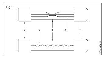
A fuse opens the circuit by blowing out when current (overload) flows in the circuit to prevent severe damage to the accessories.
