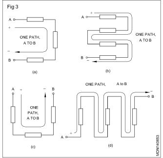
In an actual circuit diagram, a series connection may not always be as easy to identify as those in the figure. For
