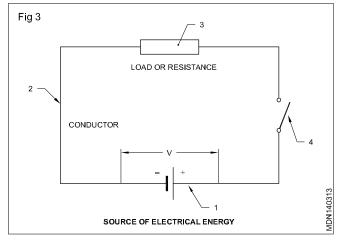
A simple electric circuit is a complete pathway of the current flow from the battery via the switch and load and back to the battery. An electric circuit consists of :
