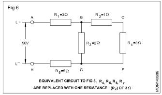
7) Combine  $R_2$  and  $R_c$  and call the equivalent resistance  $R_d$ .
