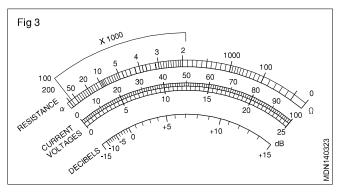
The scale for resistance measurement is non-linear. That is, the divisions between zero and infinity  $(\alpha)$  are not equally spaced. As you move from zero to the left across the scale, the division become closer together.
