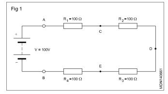
The total resistance of the circuit in (Fig 1) would be equal to  $R_{\tau} = 100 + 100 + 100 + 100 = 400$  ohms.
