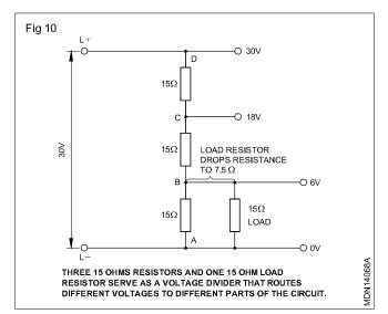
However, as soon as another resistor (load) is added as in (Fig 10), there is a further change. The load resistor serves to drop the total resistance of the lower part of the voltage divider. Use this formula for finding the equivalent resistance ( $R_{eq}$ ) of resistors of equal value in a parallel circuit:
