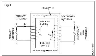
Laminated steel core transformers are used in power applications. As shown in Fig 1, the current flowing in the coil connected to the AC source is called the primary winding or simply primary. The primary is the input to a transformer. It sets up the flux in the core, which varies periodically both in magnitude and direction. The flux links the second coil, called the secondary winding or simply the secondary.
