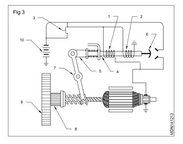
Function of solenold switch: When the starter switch (3) is turned, current flows from the battery to the solenoid windings (1) and (2). This energises the windings which pull the plunger (5). The plunger (5) operates are shift lever (7) to engage the pinion (8) on the flywheel ring gear (9). Then it closes the circuit between the battery (10) and the starting motor.
