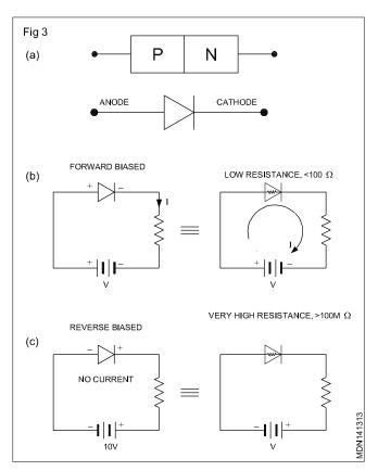
terminals one on the P side and the other on the N side are attached. Such a PN junction with terminals attached is called a **Diode**. The typical symbol of a PN-junction diode is shown in Fig 3a.
