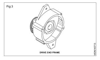
The drive end frame supports a pre - lubricated sealed sliprimgs in which the drive end of rotor shaft rotates.
