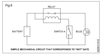
In the mechanical NOT circuit, the light bulb does not go on if switch A is closed. When switch A is opened the relay closes and the bulb is turned on.
