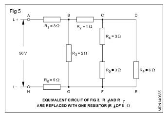
$$\frac{36}{12} R_c = \frac{R_a \times R_b}{R_a + R_b} = \frac{6 \times 6}{6 + 6}$$
