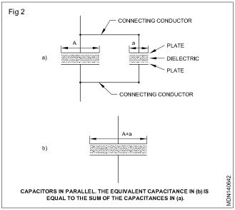
**Example:** Suppose three capacitors are connected in parallel, where two have a breakdown voltage of 250 V and one has a breakdown voltage of 200 V, then the maximum voltage that can be applied to the parallel group without damaging any capacitor is 200 volts.
