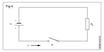
**Short circuit:** A short circuit will occur when two terminals of the same circuit touch each other. A short circuit may also occur if the insulation between the two cores of the cable are defective. This results in a lower resistance. This causes a large current to flow which can become a hazard.
