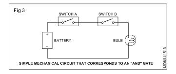
Similarly, in an actual AND gate, there will be an "on" signal (often represented as the number 1) at the output terminal (C) only if there is a voltage at both input terminals (A and B). If either A or B is zero (off) or if both are zero, C will also be zero. These combination can be shown in a truth table.
