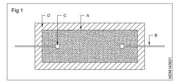
A mixture of finely powdered carbon or graphite(A), filler and binder is made into rods or extruded into desired shapes. Leads(B) made of tinned copper are then attached to the body either by soldering or embedding(C) in the body. A protective layer/tube(D) of phenolic or Bakelite is moulded around the assembly. Finally its resistance value is marked on the body.
