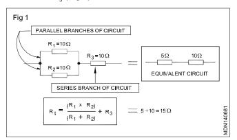
Thus,  $R_1$  and  $R_2$  form the parallel component, and  $R_3$  the series component of a series-parallel circuit. The total resistance of any series-parallel circuit can be found by merely reducing it into a simple series circuit. For example, the parallel portion of  $R_1$  and  $R_2$  can be reduced to an equivalent 5-ohm resistor(two 10-ohm resistors in parallel).
