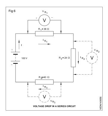
When Ohm's law is applied to the complete circuit having an applied voltage V, and total resistance R, we have the current in the circuit as
