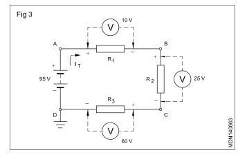
Trace the complete circuit in the direction of current from the + terminal of the battery to A, A to B, B to C, C to D, and D to the negative terminal. Mark plus (+) where the current enters each resistor and minus (–) where the current leaves each resistor.
