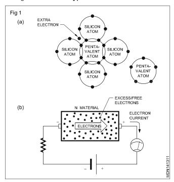
When a N-type material is connected across a battery, as shown in Fig 1b, current flows due to the availability of free electrons. As this current is due to the flow of free electrons, the current is called electron current.
