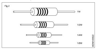
The physical size of a resistor should be sufficiently large to dissipate the heat generated. The higher the physical size, the higher is the heat that a resistor can dissipate. This is referred to as the power rating or wattage of resistors. Resistors are manufactured to withstand different power ratings.
