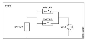
If there is voltage at either input terminal (or if there is a voltage at both inputs) there will be voltage at the output terminal "OR" gate truth table is given.
