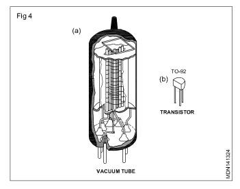
Compared with the present day transistors the vacuum tubes were big in size, consumed more power, generated lot of unwanted heat and were fragile. Hence vacuum tubes became absolute as soon as transistors came to market.
