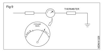
Thermistors can also be used to detect the temperature of the air. Many of the computer controlled fuel system in use utilize air temperature as an input. These are easily installed and wired into the computers and will have their resistance changes seen as temperature changes.
