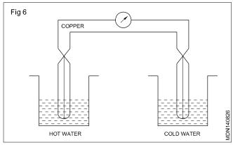
This is such an arrangment where circuit is closed by wires of different metals. One metal wire is kept at low temperature and the other at high temperature. In this way thermo-electro motive force is created which can be seen by galvanometer. This works on the effect of seebake.
