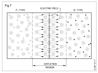
There is a layer of positively charged ions on the N-side and on the P-side of the junction there is a layer of negatively charged ions. An electric field is created across the junction between the oppositely charged ions. This is called a junction field. The junction field is also known as 'barrier'. The distance between the sides of the barrier is the 'width' of the barrier.
