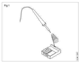
Inspection of soldering iron: Most soldering irons are powered by AC main voltage. This voltage level is high and can give shock if one is careless. Soldering irons will generally have lengthy mains cable. While using the iron, the mains cable gets twisted and will have to bear physical stain. Because of this strain, the insulation of cable may get cut. This may lead to live wires protruding out. The live wires give severe electrical shocks if it touches the user.
