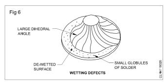
Wetting defects are easily recognised by the inability of the solder to cover all the metal surfaces at the joint and the formation of a large dihedral angles as in Fig 6.
