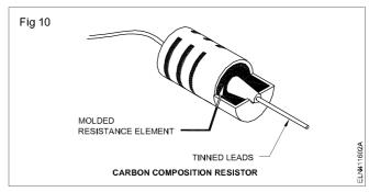
Carbon resistor are available in values of 1 ohm to 22 megohms and of different power ratings, generally 0.1, 0.125, 0.25, 0.5 and 2 watts.
