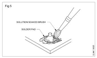
When the residue has been dissolved, dry the joint with a lint-free cloth to remove as much of the dissolved residue as possible.
