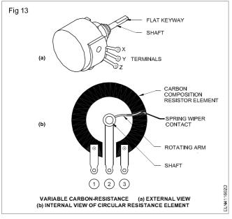
It is provided with 3 terminals as shown in Fig 13 and 14. They are available with carbon tracks (Fig 13) and wire wound (Fig 14) types. Trimmer potentiometers (or) resistor which can be adjusted with the help of a small screw driver. (Fig 15).
