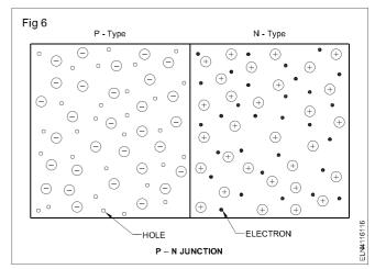
The free electrons in the N-regions diffuse across the junctions into the P-region. The free electrons lose energy and recombine with the holes in the P-regions. This recombination eliminates a free electron and a hole. When the electron moved from the N-region and diffused across the junction, it leaves the atom to be a positive ion.
