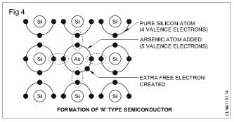
Because the outer orbits of the atoms can hold eight electrons, no hole is available for the fifth electron in the arsenic atoms to move into. It, therefore, becomes a free
