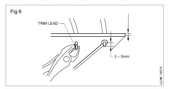
After cutting the excess lead length, the component lead must be bend and terminated, on PCB.
