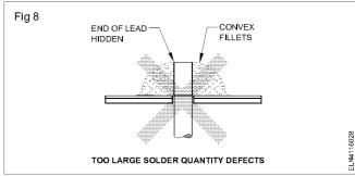
**Mechanical defects**: Mechanical defects of a solder joint are caused by;
