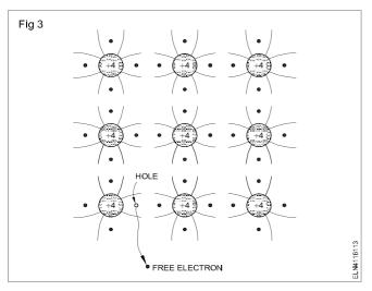
When an electron breaks a covalent bond and moves away, a vacancy is created in the broken covalent bond. This vacancy is called a 'hole'. A hole has a positive charge. When a free electron is liberated, a hole is created.
