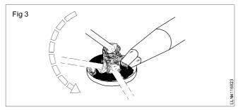
Continue applying the solder to the joint until complete wetting of the joint has been achieved and the joint has a concave fillet as in Fig 4
