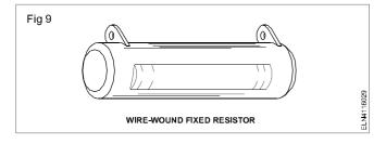
One type of Wire-wound resistor is called as fusible resistor enclosed in a porcelain case. The resistance is designed to open the circuit when the current through it exceeds certain limit.
