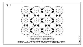
The union of atoms sharing the valence electrons is called a **covalent band**. That means a valence electron being shared by two adjacent atoms. Each atom appears to have a full outer shell of eight electrons.
