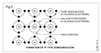
A hole is created in the place of the eighth electron. Now that the number of holes exceeds the number of free electrons the substance becomes 'P' type material. The holes in P-type are the **majority** carriers, and the free electrons are the minority carriers.
