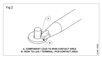
Slowly feed the solder into the joint starting close to the soldering tip and moving towards the edge of the joint as in Fig  $3\,$
