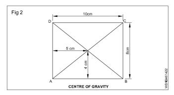
3 A thin lamina is shown in the figure below. Find the centre of gravity.
